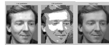
Fig 5 Bit quantized images: 2bit, 4 bit and original image of 8 bits
